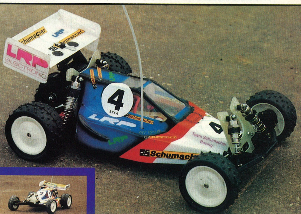
Kevin Moore's Cougar with modified shock absorber towers.
